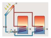
S1 sensor for supply line S4 sensor for return line S13/5V flow sensor
