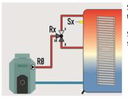
Sx sensor for top of storage Rx N tank
