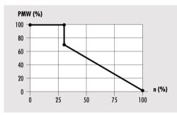
PWM (%) – inverted PWM signal n (%) – pump speed sent by the controller
