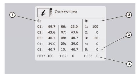
If flex 400 modules are connected, a menu item with an overview of the inputs and outputs will appear for each of these modules.
