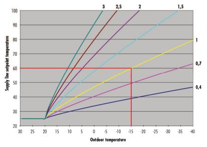
The example graphic shows that when curve 1 (yellow) is selected and the outdoor temperature is -15 °C, the supply line setpoint temperature will be 60 °C.
