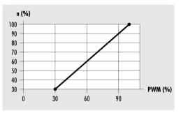
n (%) – nominal speed of the pump PWM (%) – non-inverted PWM signal
