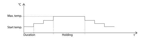
The number of steps is calculated from the difference between the start temperature and the maximum temperature and from the increment.
